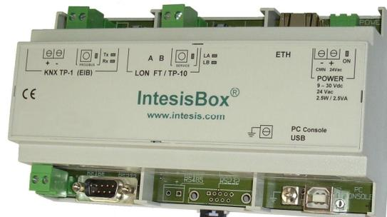
Gateway for monitoring and control KNX EIB installations from LonWorks based control systems (TAC, Kiebak & Peter...)
