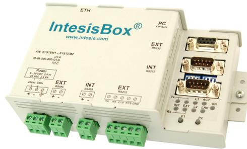
Gateway for monitor and control of VRV air conditioning systems of the main manufacturers from Modbus (RTU or TCP) master or client devices (SCADA, BMS, PLC, HMI, TouchPanels...), and in general to monitor/control any LON (TP/FT-10) system or device from Modbus.
