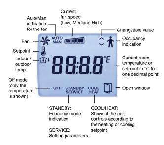
The display is handled using the buttons on the thermostat:
