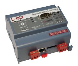
L-INX Automation Servers LINX-210 and LINX-211 are controllers for automation tasks in BACnet networks. The powerful Automation Servers provide connectivity features to integrate into BACnet networks, where the L-INX Automation Servers represent BACnet Building Controllers (B-BC). The LINX-211 adds a built-in BACnet/IP Router with BBMD and slave proxy functionality.
