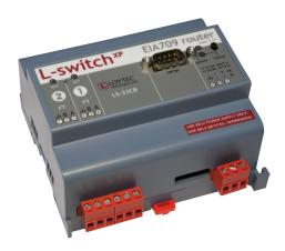
The L-Switch<sup>XP</sup> is the solution for interconnecting multiple 2-wire channels (TP/FT-10 or TP/XF-1250 channels) in LonMark Systems. It provides up to five ports and routes packets between these ports. The L-Switch<sup>XP</sup> router delivers first class performance and flexibility in use. In order to provide the optimal router configuration, the L-Switch<sup>XP</sup> comes with 2 to 5 ports as well as the two operating modes "Smart Switch Mode" and "Configured Router Mode".
