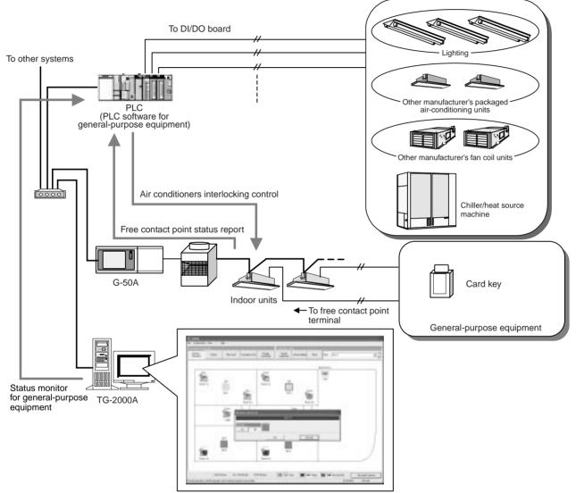
Figure 11-1 Configuration of the general-purpose control system
