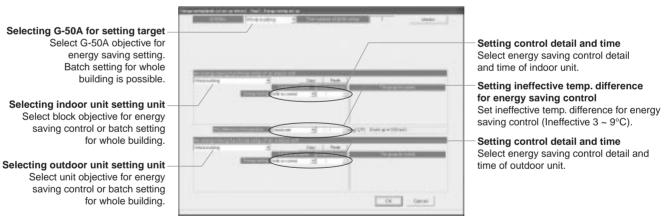
Figure 9-2 TG-2000A energy saving control setting screen
