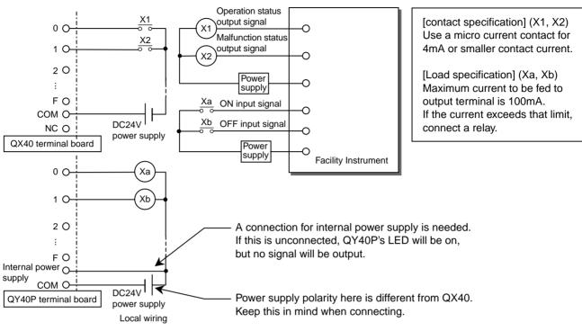
Figure 12-6 General-purpose control terminal connection diagram
