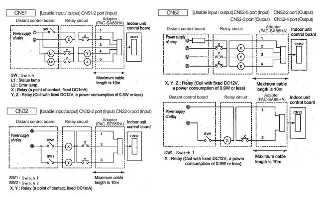
Figure 11-5 Free contact point (input 3, 4, output 1, 2, 3) connection diagram
