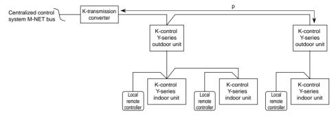
Figure 4-5 K-control Y-series wiring example
