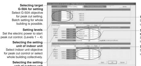
Setting control detail and time Select the detail and time of indoor unit peak cut control.
