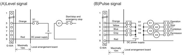
\* Special local arrangements are required for the relay, DC power supply (DC 12V, or DC 24V), and extension cables, etc.
