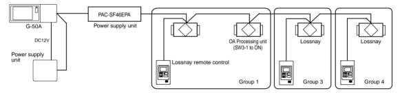
Figure 5-3 Electricity supply using a Lossnay system
