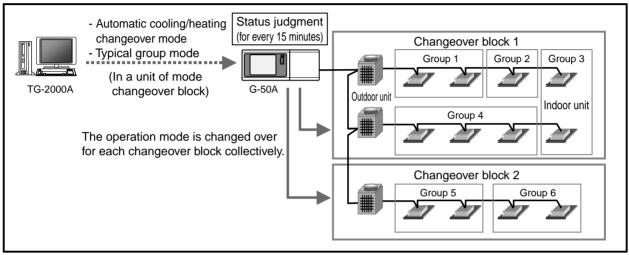
Figure 16-1 Configuration of auto-changeover system
