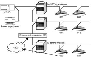
Figure 5-8 K-control converter address
