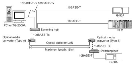
Figure 13-8 Chart of LAN system using optical cable
