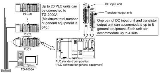
Figure 12-5 Restriction on the number of PLC units for multi-purpose control functions
