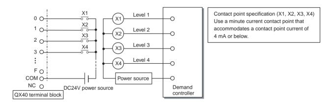
Figure 12-8 Demand controller terminal connection diagram
