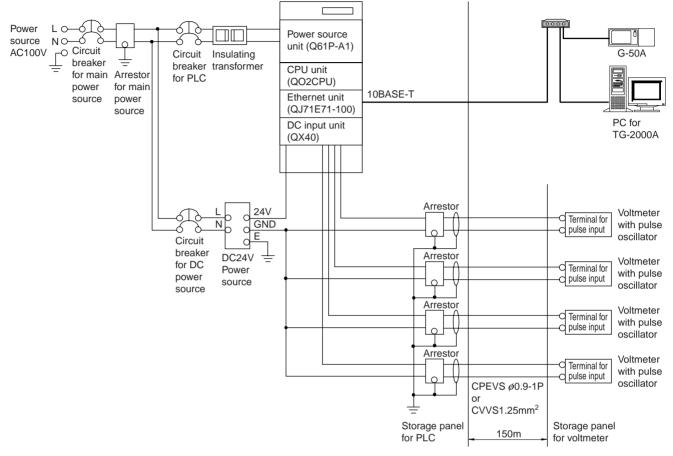
Figure 12-9 Wiring example around PLC
