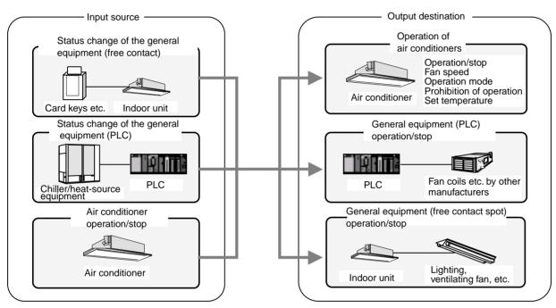
\*If "air conditioner operation/stop" is selected as the input source, "operation of air conditioners " cannot be selected as the output destination.
