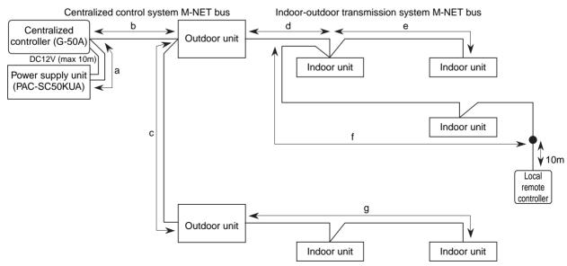
Figure 4-1 M-NET bus wiring diagram
