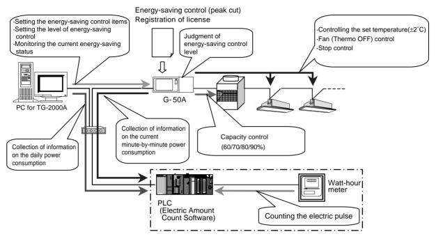
Figure 9-5 Configuration of the system using the power consumption monitoring method
