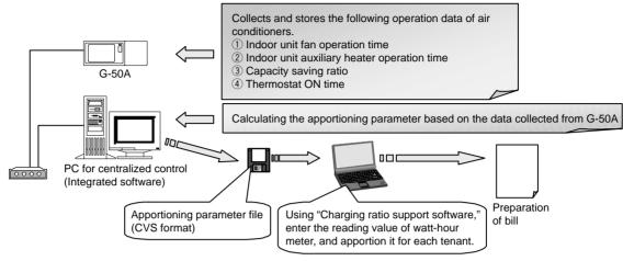
Figure 8-12 Mechanism of electric power manual input
