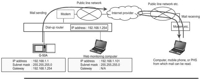
\* [192.168.1.254] is recommended for the IP address of the dial-up router. Refer to the dial-up router instruction manual for the setting method of the IP address.
