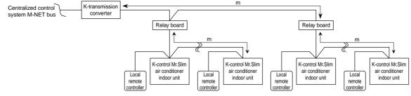
Figure 4-4 Relay board wiring example
