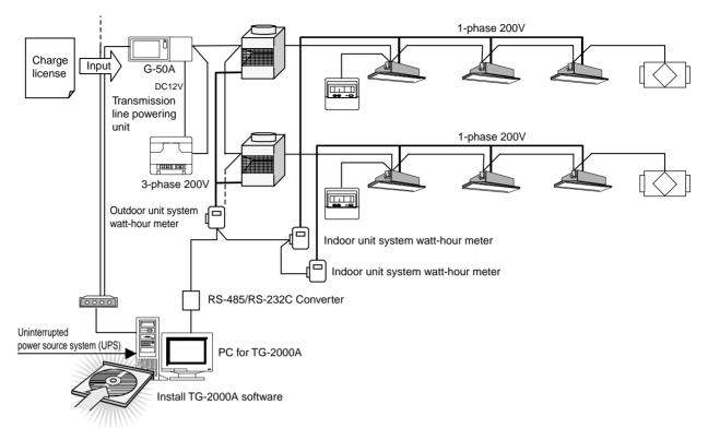
Figure 8-10 Basic configuration of power consumption PC direct reading system (RS-485 Watt-hour meter)
