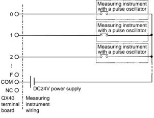
Figure 12-3 QX40 terminal connection diagram
