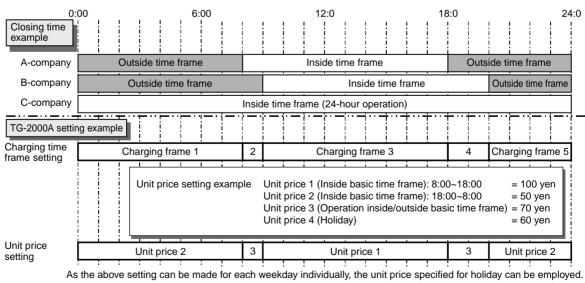
Figure 8-14 Setting example of charging time frame and unit price
