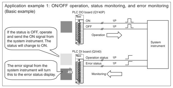
\*When the system instrument does not provide the output of operation status, connect to the input of operation status by installing a selfholding circuit.
