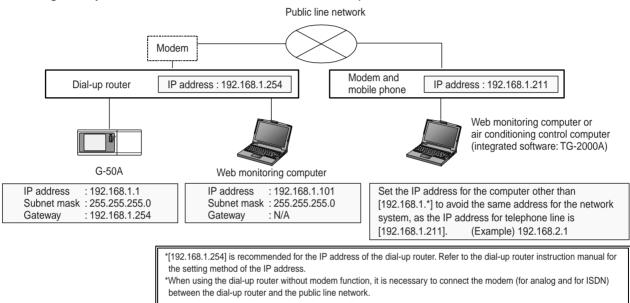
Figure 6-3 Remote monitoring system setting example
