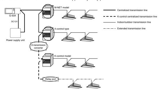
Figure 5-2 Transmission line supply classification
