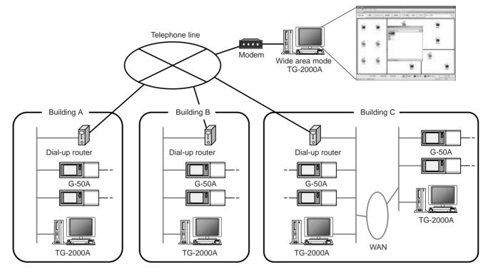
Figure 2-4 Wide area monitoring system example
