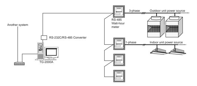
Figure 10-2 Outline wiring of measuring instruments
