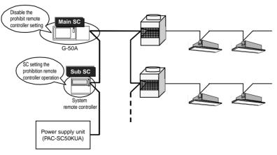
Figure 5-1 System controller concept
