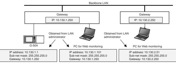
Figure 13-2 Setting example 1 of existing LAN system
