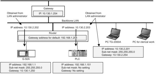
Figure 13-3 Setting example 2 of existing LAN system
