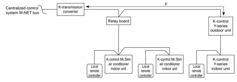
Figure 4-6 K-control mixing system example
